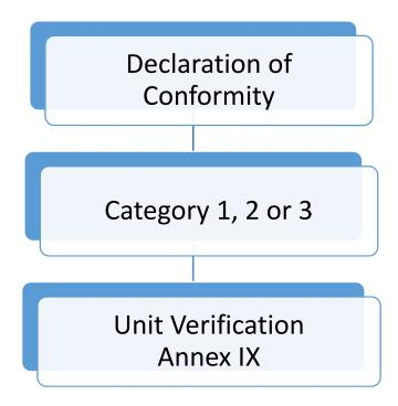
Unit Verification combines all of the requirements of the testing, assessment and quality control assessment into one certificate. It is used for single items or small numbers of items. The Notified Body verifies the quality of the manufactured product, so the Notified Body number is included next to the CE mark, even for equipment that does not normally need it (Category 3)
