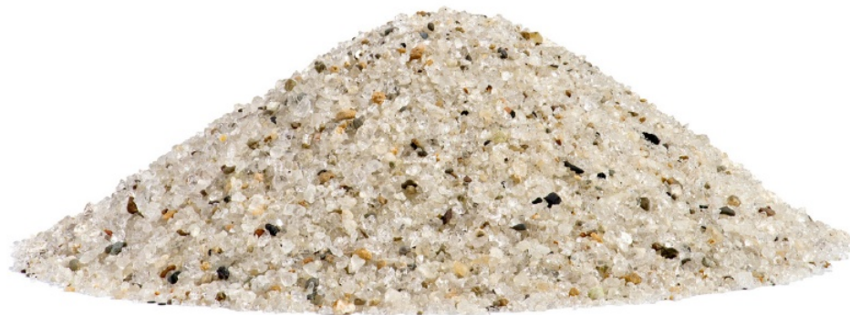
The glass sand must have particles within a certain size range, and also has to pass an electric strength test which uses two parallel plates – Image: Shutterstock
